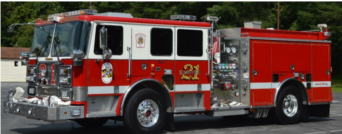
Example of short wheelbase engine with 750-gallon water tank
