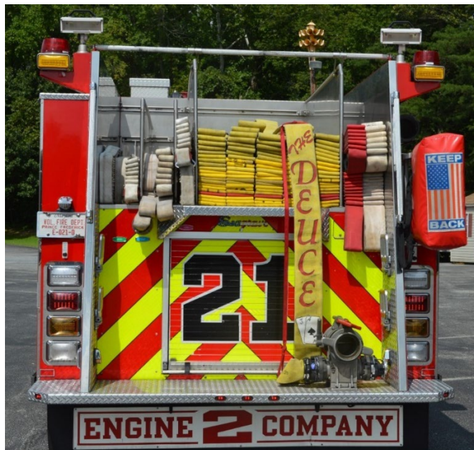
Example of low rear hose bed with 750-gallon water tank
