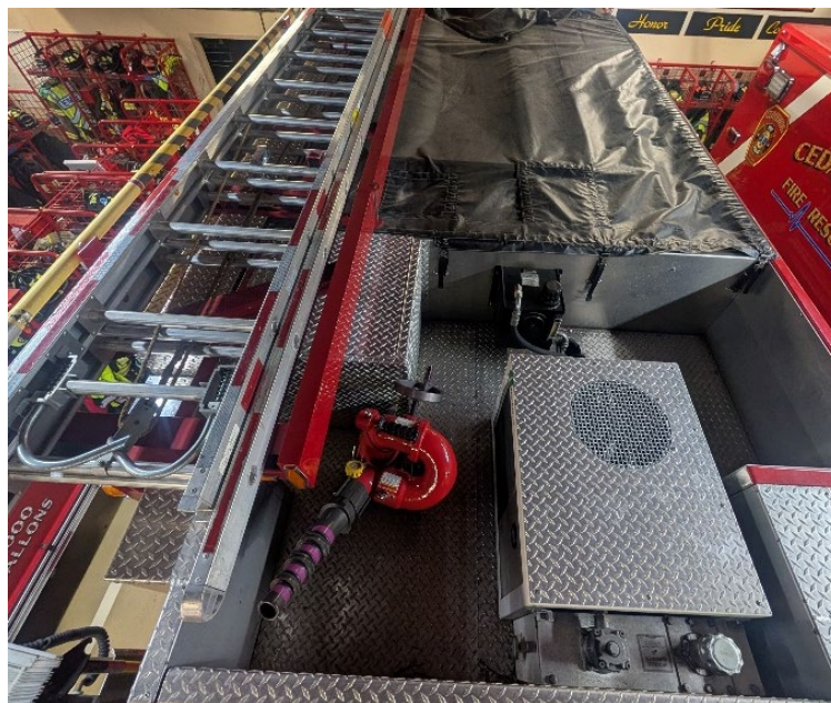
The master stream device is not easily accessible and dangerous
