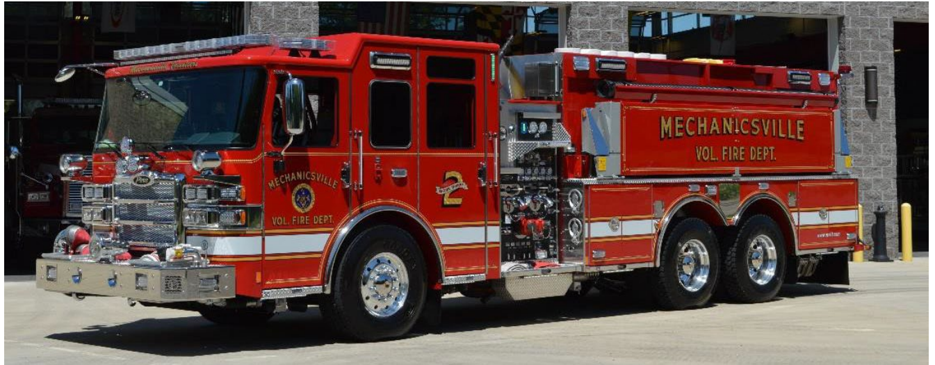
Example of a short wheelbase engine with a 2000-gallon water tank
