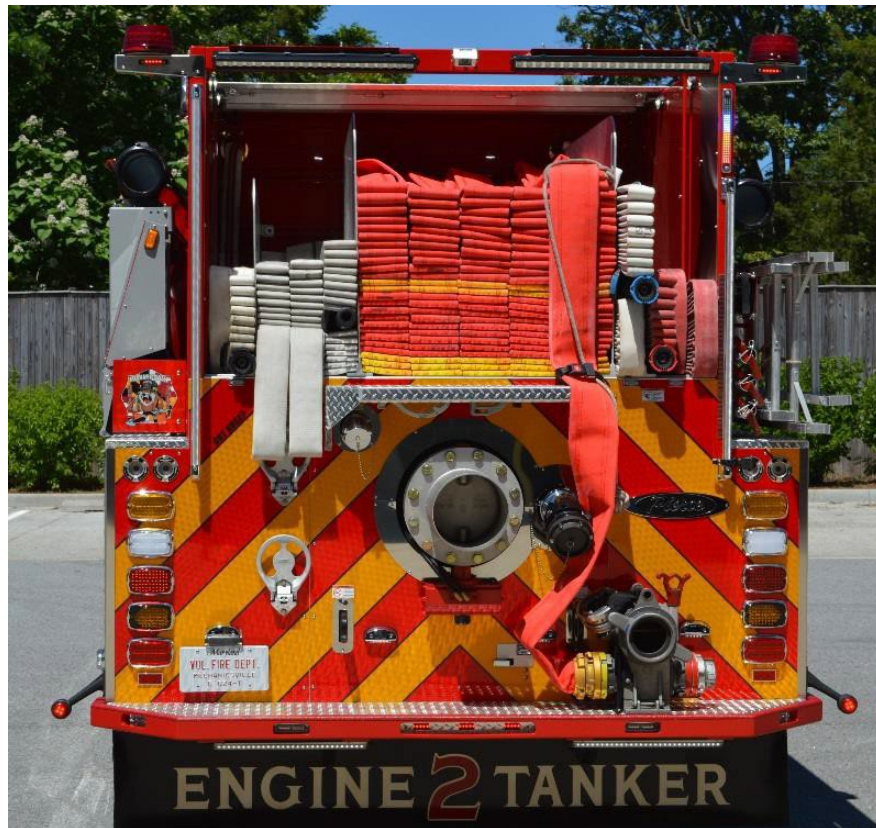
Example of a low rear hose bed with a 2000-gallon water tank
