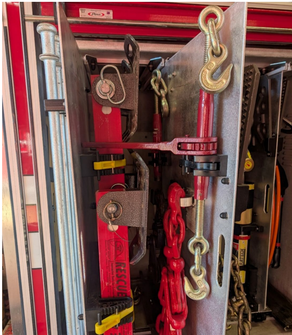
Equipment on slide trays is mounted too close to one another. The equipment is knocking other equipment when the slide tray is deployed.
