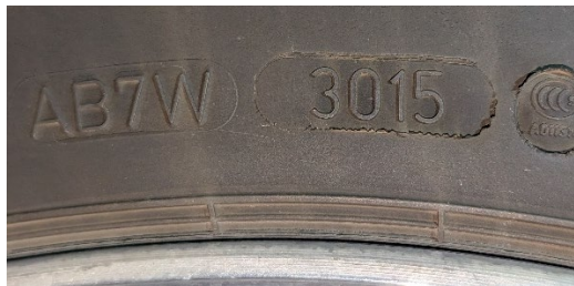
Rear tires are 2015 and are out of date and need to be replaced.
