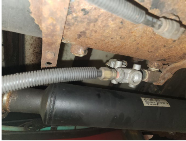
Bolt-on Components Rusting
