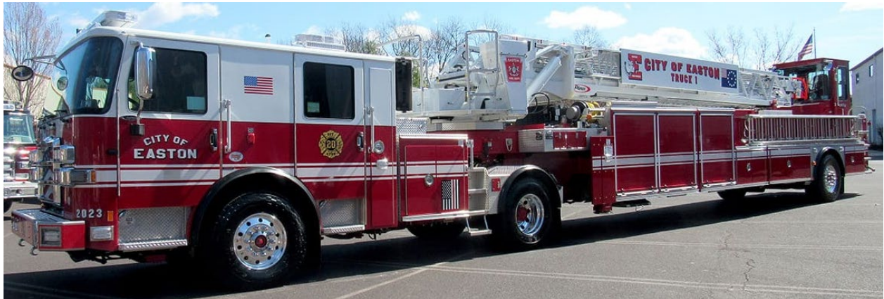
This TDA would meet the needs of the Cedarburg Fire Department. It measures 59' 6" long and is 11' 2" tall and would fit in Cedarburg Station 1.
