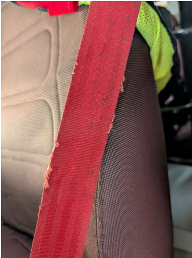
The driver's seatbelt is frayed and needs to be replaced.
