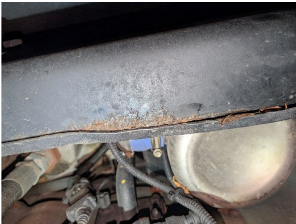
Frame rails showing signs of rust and corrosion behind the liner.
