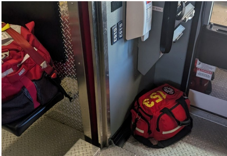
Loose Equipment in the seating area needs to be secured in 9G rated brackets.
