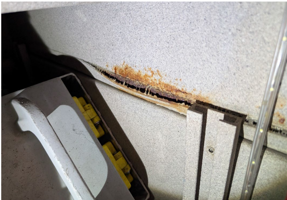
Major corrosion damage, bulging, and stress damage to the rear compartment under the rear hose bed.
