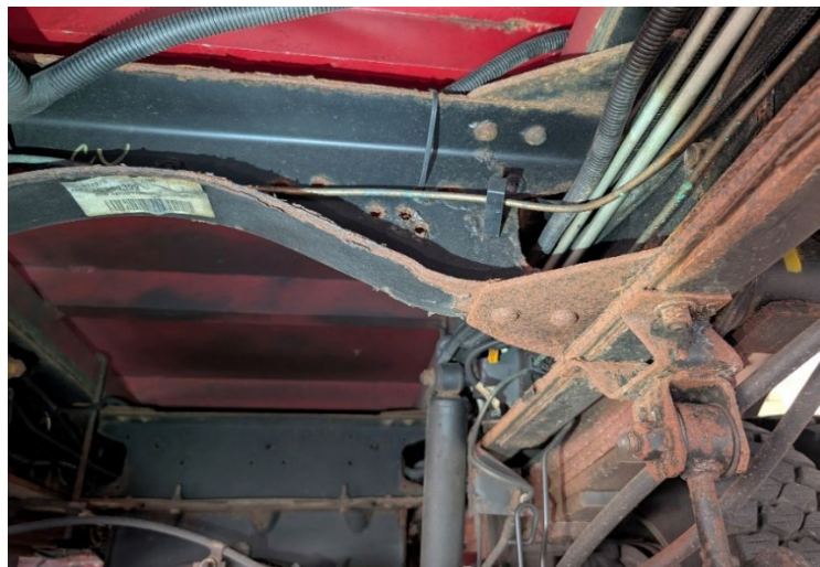
Rust on the underside of the vehicle
